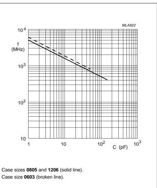
Fig.6 Series resonance frequency as a function of capacitance.
